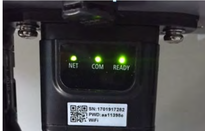
Figure 89 - Final status of LEDs
