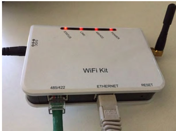
Figure 92 - Ethernet cable connected to the datalogger
