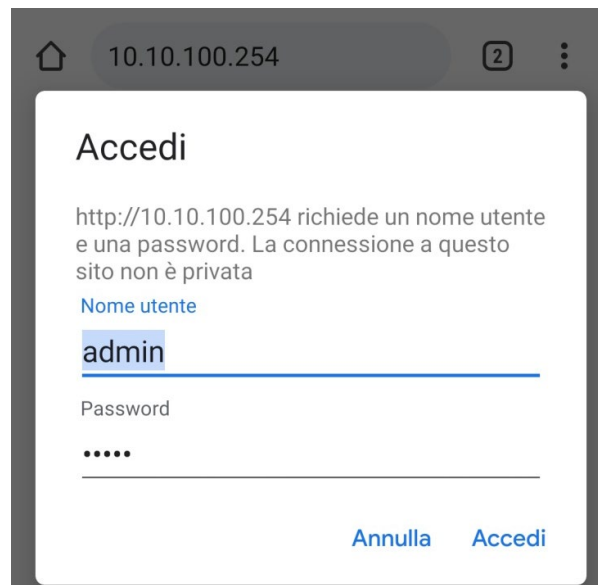
Figure 167 - Screen for accessing the web server to configure the datalogger
