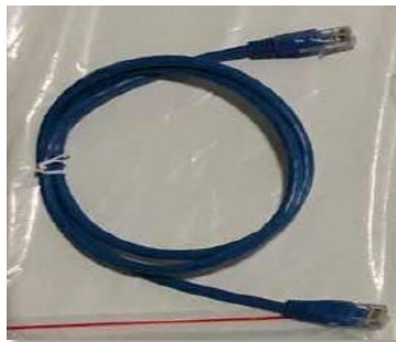
Figure 50 – Communication cable between WeCo 5k3 batteries
