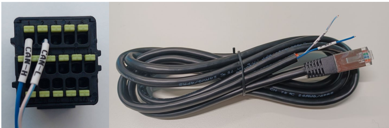
Figure 13 - Pylontech communication cable to be inserted into the battery communication input
