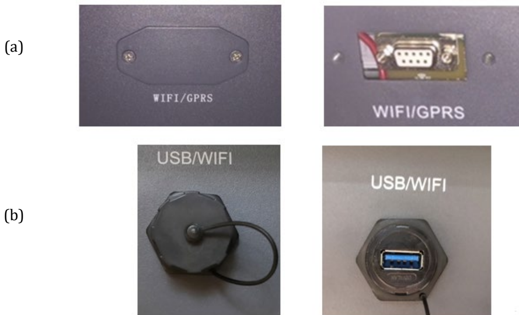
Figure 114 - Slot for external Wi-Fi adapter
