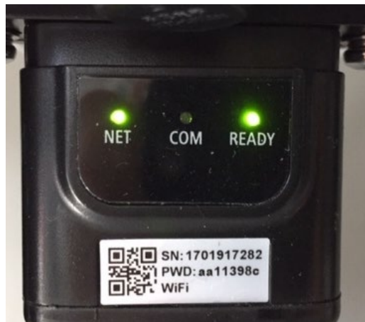
Figure 144 - Irregular communication status between inverter and adapter
