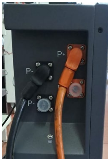
Figure 85 – Terminal block of the AZZURRO ZSX 5120 battery
