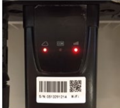
Figure 133 - Irregular communication status between inverter and Wi-Fi
