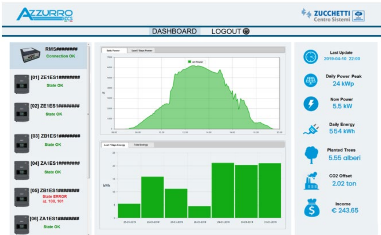
Figure 180: Example of local monitoring page
