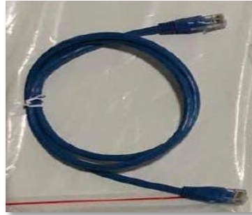
Figure 79 – Communication cable between AZZURRO 5000 PRO batteries
