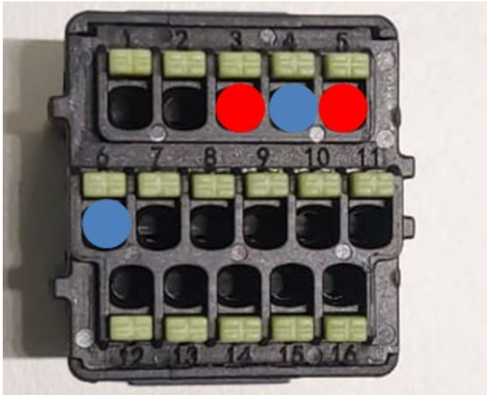
Figure 159 – Connecting the serial line via the communication connector for 3PH HYD5000-HYD20000-ZSS inverters
