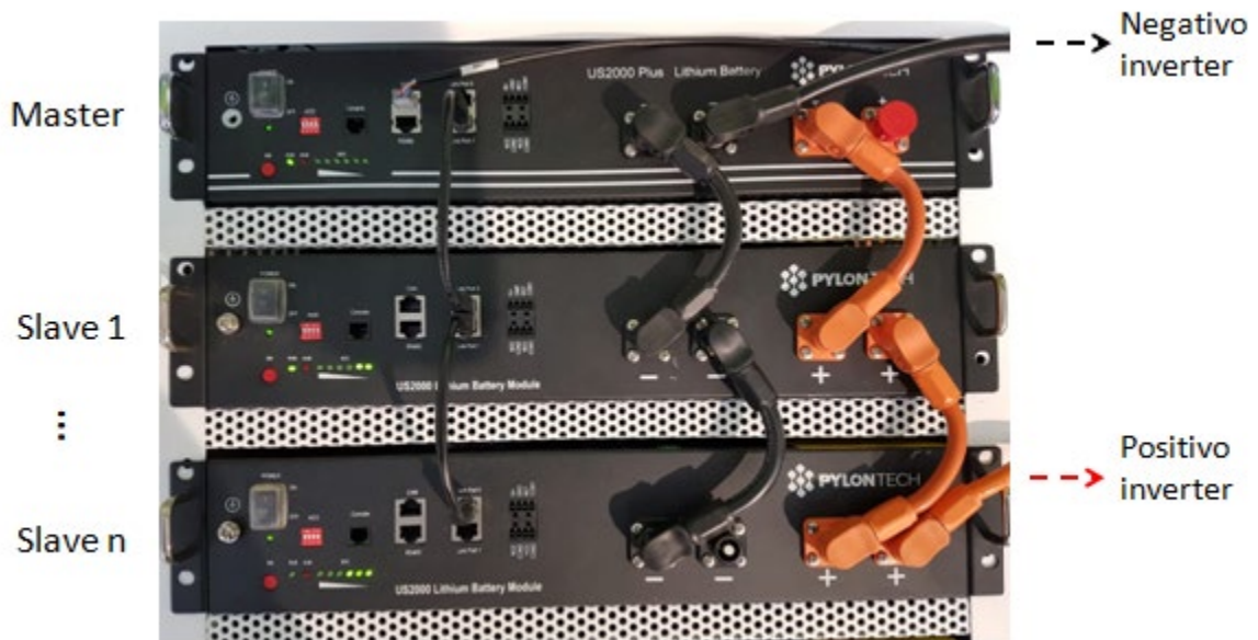
Figure 17 - Connecting three Pylontech batteries in parallel
