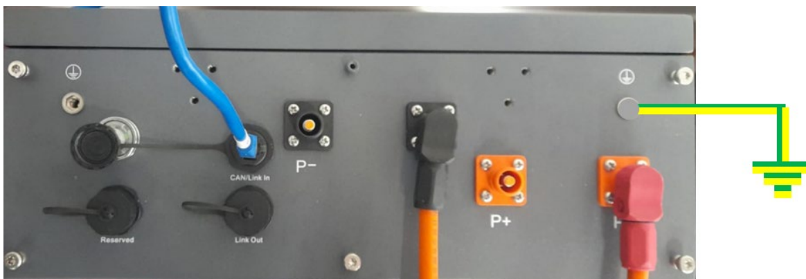
Figure 94 – Terminal block of the AZZURRO 5000S battery
