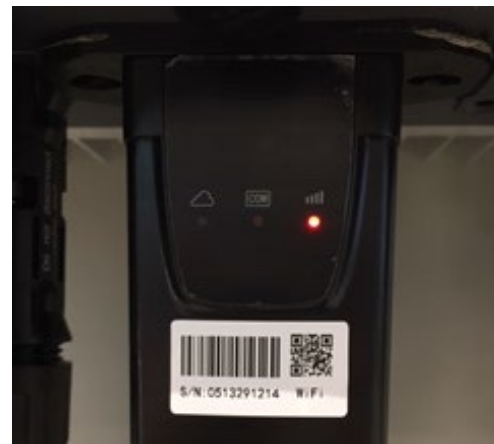
Figure 135 – Irregular communication status between Wi-Fi and remote server
