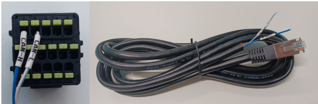
Figure 75 - Communication cable between the inverter and AZZURRO 5000 PRO battery
