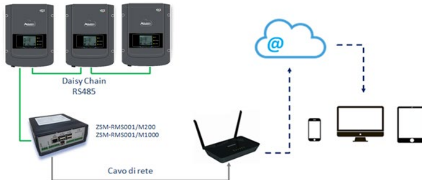
Figure 153 – Diagram for the functioning of the ZSM-RMS001/ M200 / ZSM-RMS001/M1000 datalogger
