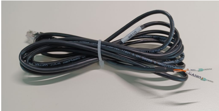
Figure 23 - Communication cable between the inverter and WeCo 4k4 battery
