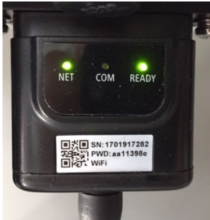
Figure 133 - Irregular communication status between inverter and Wi-Fi
