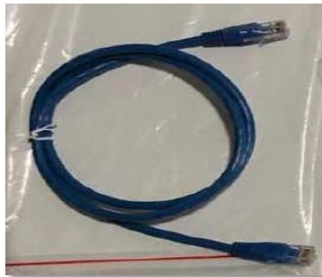
Figure 57 – Communication cable between WeCo 5K3XP batteries
