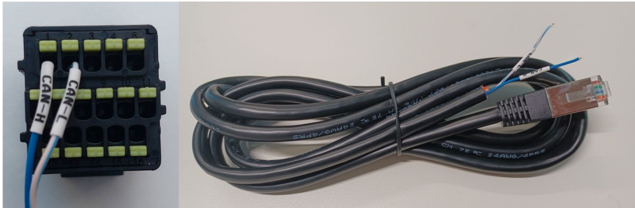
Figure 83 - Communication cable between the inverter and AZZURRO ZSX 5120 battery
