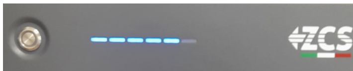
Figure 95- Power button of the AZZURRO 5000S battery
