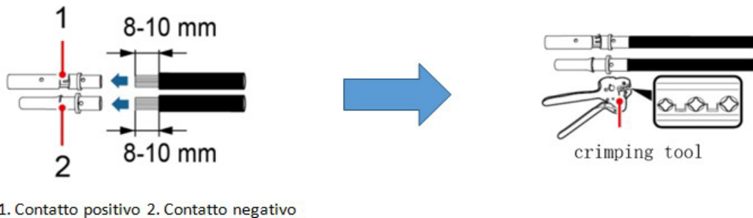
Figure 9 - Preparing the positive and negative PV cables
