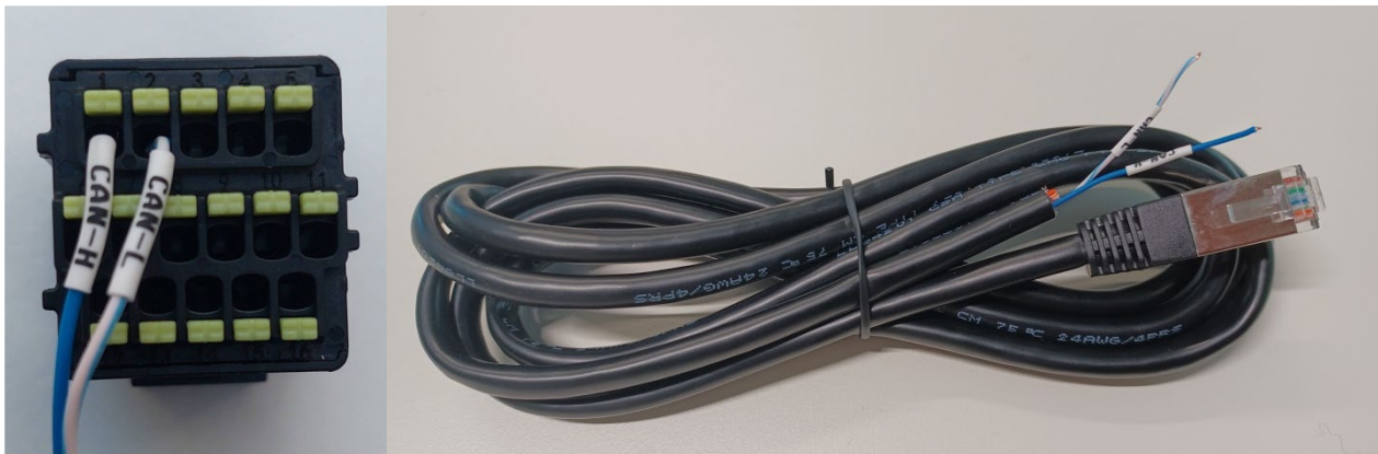
Figure 18 - Pylontech communication cable to be inserted into the battery communication input
