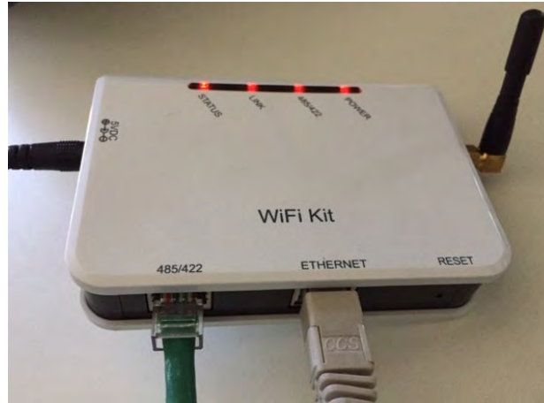
Figure 82 – Ethernet cable connected to the datalogger
