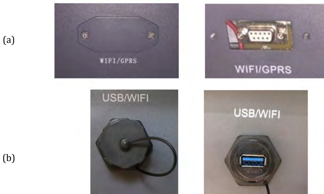
Figure 66 – Port of the 4G adapter
