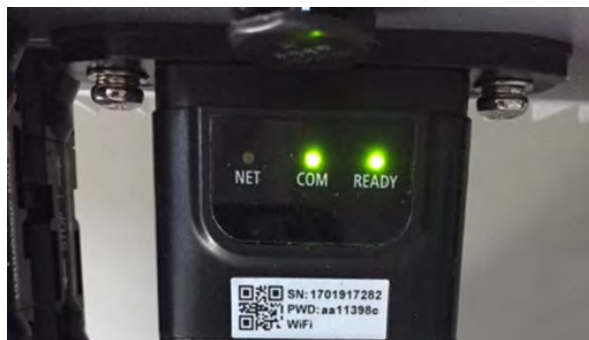
Figure 68 – Initial status of LEDs
