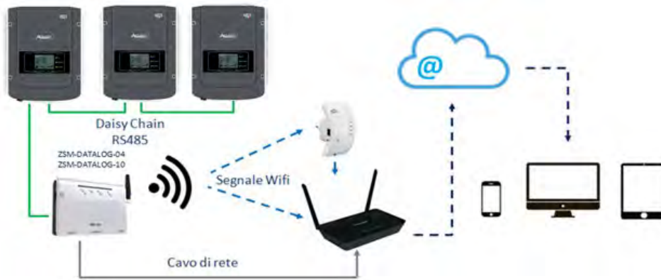
Figure 72 – Diagram for connecting the ZSM-DATALOG-04 / ZSM-DATALOG-10 datalogger
