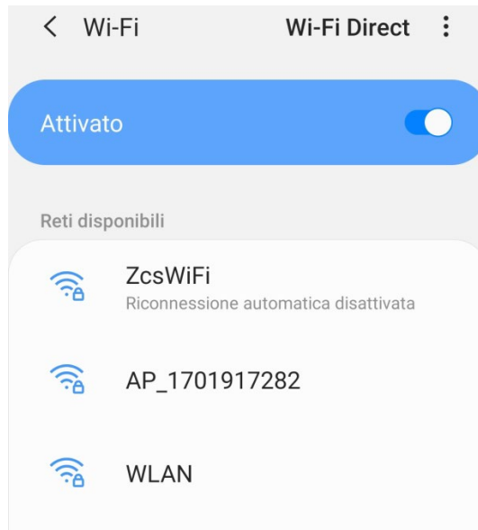
Figure 264 - Disabling automatic reconnection to a network
