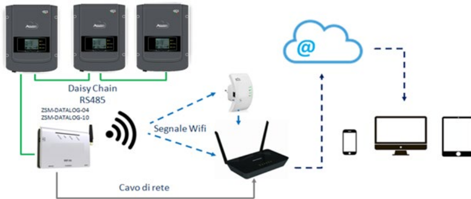
Figure 252 – Diagram for connecting the ZSM-DATALOG-04 / ZSM-DATALOG-10 datalogger
