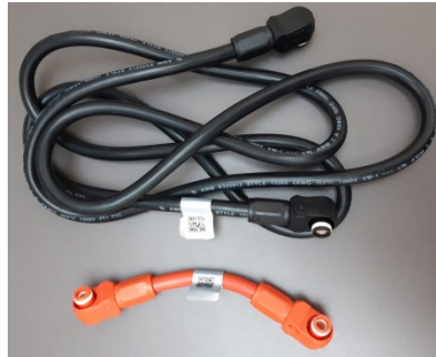
Figure 43 - Connection cables between the BMS and battery modules
