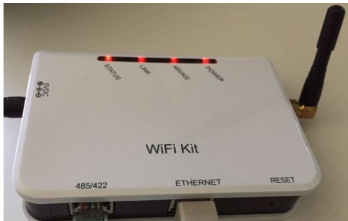
Figure 275 – LED indicating the correct configuration of the datalogger
