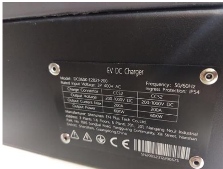
Figure 2 - Labels present on the charging station
